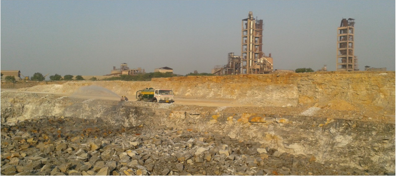
Wetting of Blasted muck pile before loading to reduce dust generation
